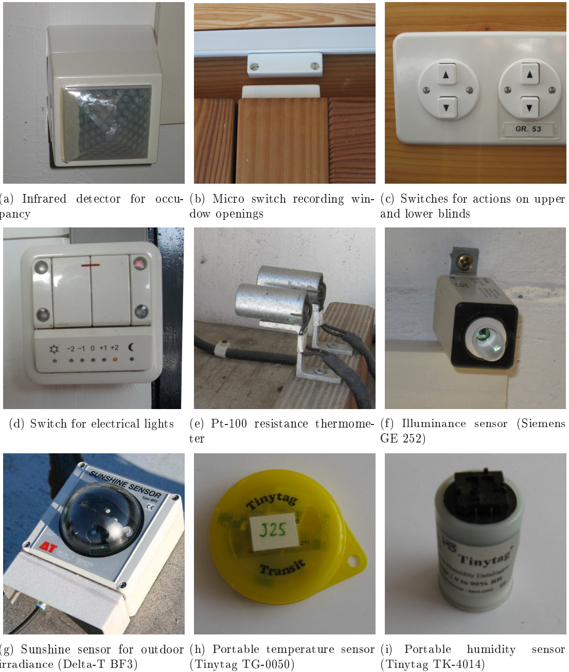
Figure 2.3: Measurement devices used in the field survey
