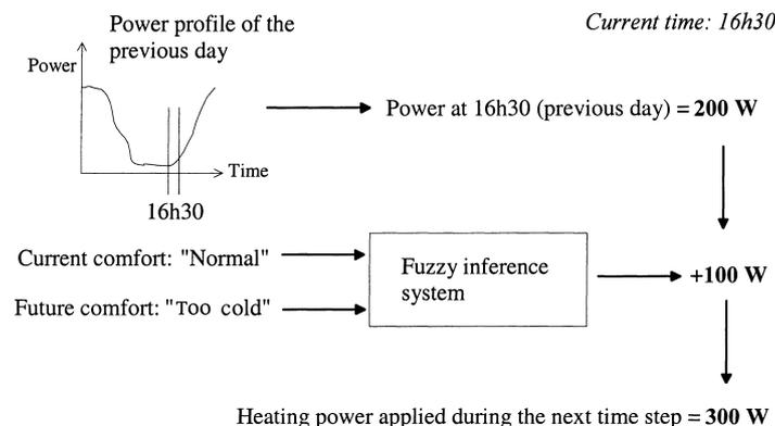
Fig. 4. Operation of the heating controller.
