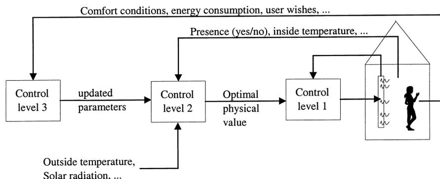
Fig. 1. Principle block diagram of the three nested control loop levels.
