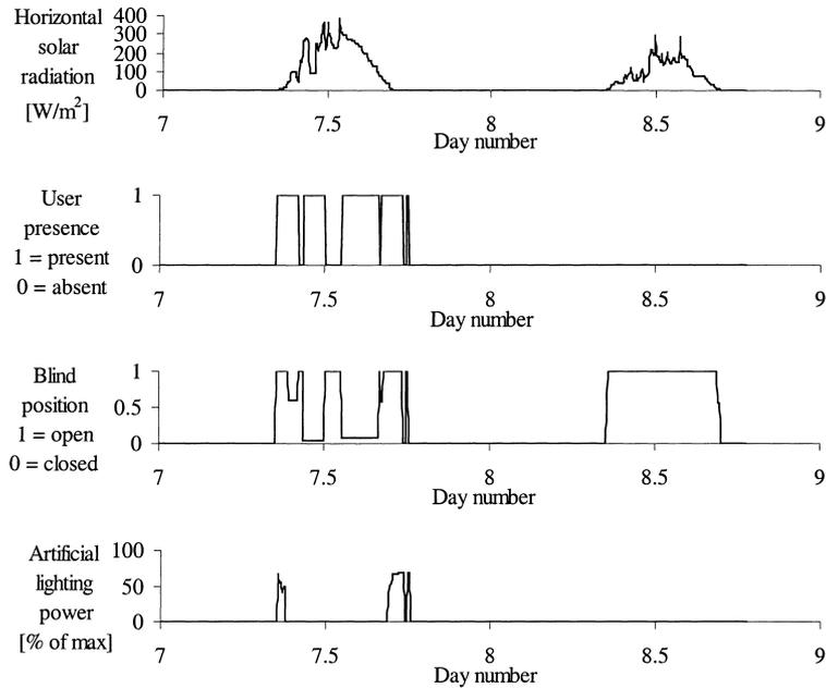
Fig. 8. Global solar irradiance, presence, blind position and artificial lighting power provided by the integrated controller. Day 8 corresponds to Saturday, 8 January 2000 at midnight.
