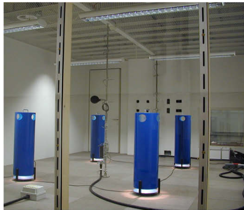
Fig. 8. HVAC-Laboratory test room equipped with TABS: external view from the laboratory hall (left) and view from the weather zone into the room (right).
