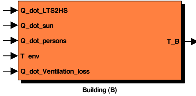
Figure 4.2.1.2: Block diagram of the building.
