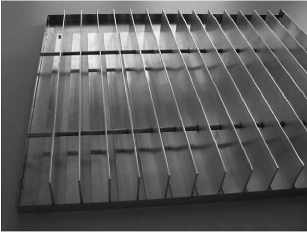
Fig. 11. Aluminum fins to increase the conductivity in the PCM/Gyp- sum-composit.
